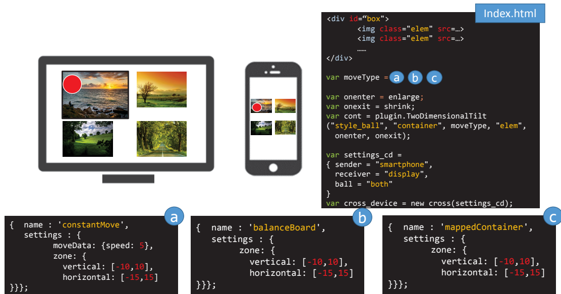
Figure 1: Example use of our framework to continuously control an indicator on a larger device via motion gestures. Developers can decide on the type of interaction by changing the moveType variable, in this case: (a) Constant Move , (b) Balance Board and (c) Mapped Container .
